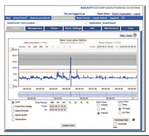
Changes in flow patterns can quickly identify emerging I&I issues to prevent spills
