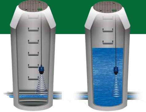
*Our Subsonic® sensor measures from the bottom of the invert to the manhole cover using both ultrasonic and pressure readings, ensuring level is measured even if the sensor is submerged*
