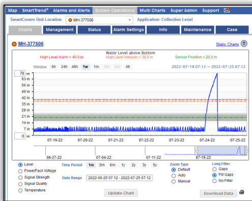
Lift Station Failure Alert
