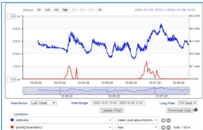
Figure 2: Water leak or inflow and infiltration
